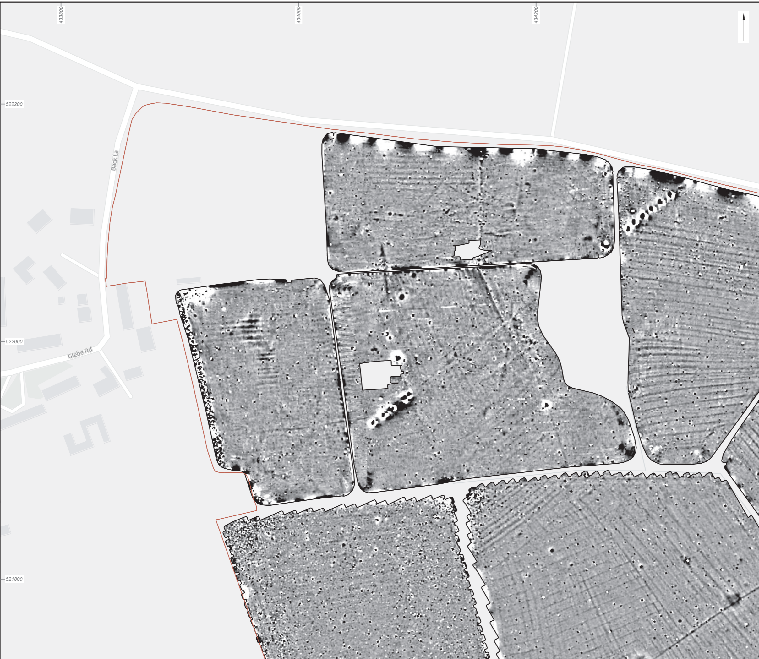
Area 3 detailed gradiometer survey results: greyscale plot
