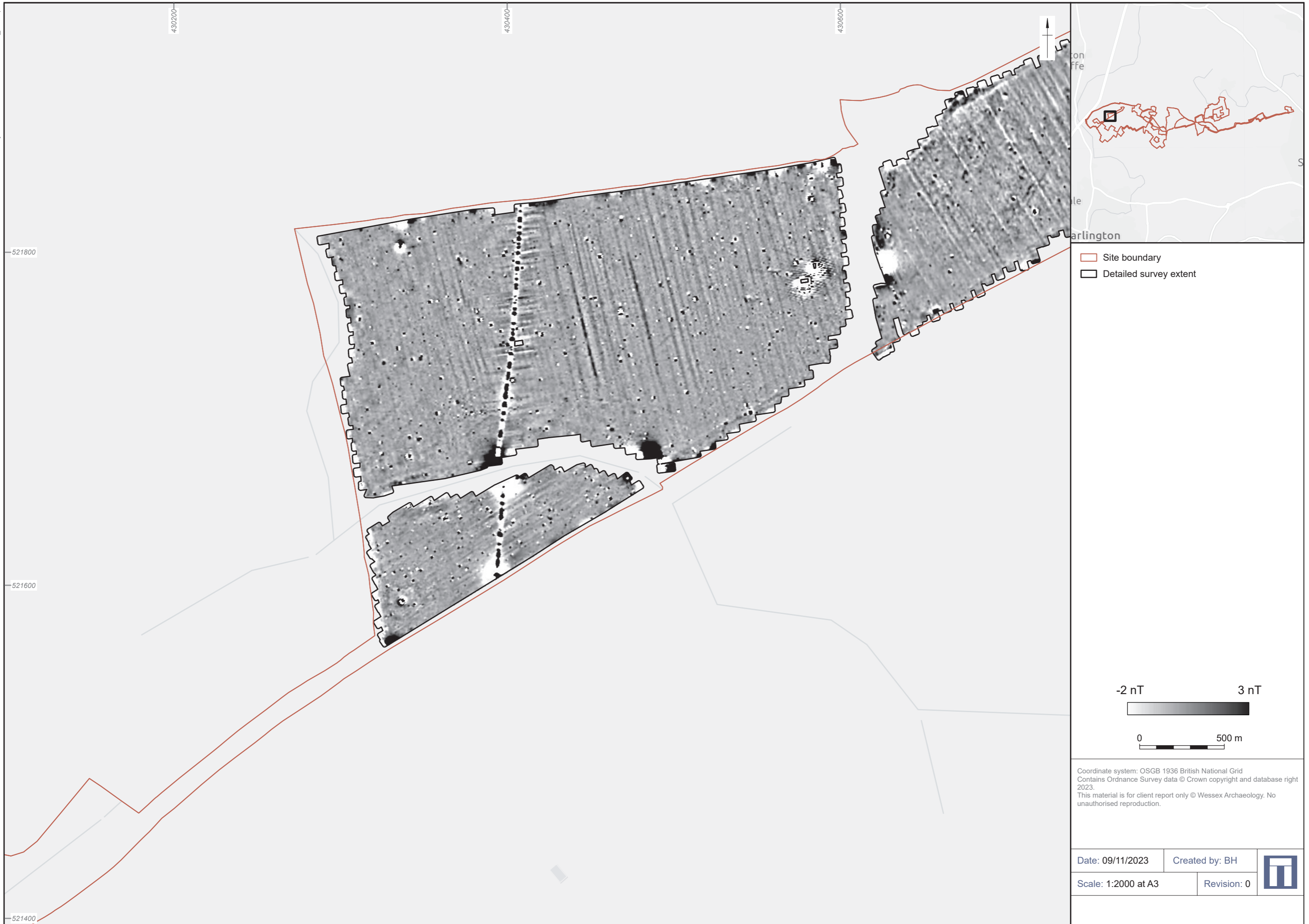
Area 1 detailed gradiometer survey results: greyscale plot
