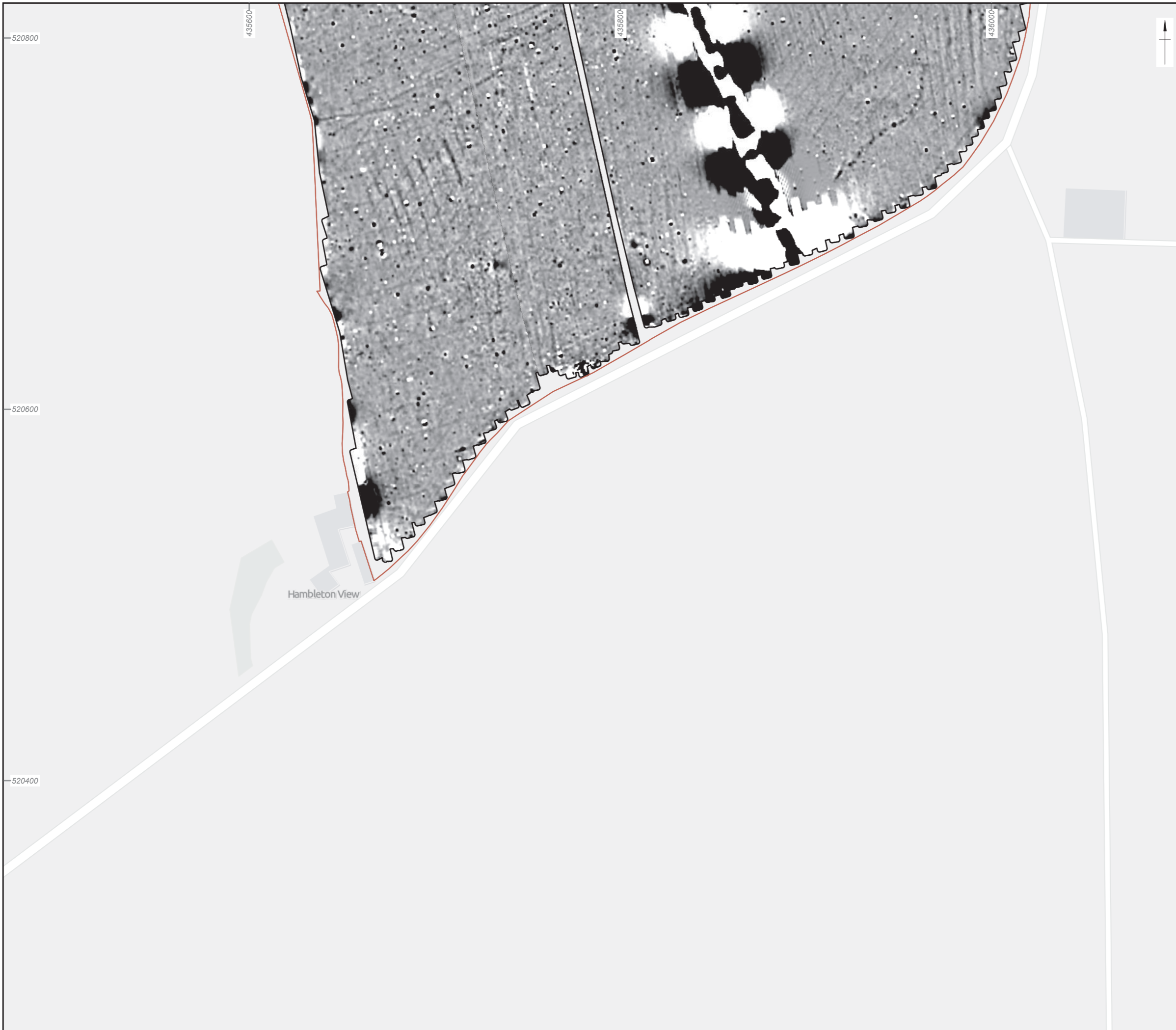
Area 3 detailed gradiometer survey results: greyscale plot
